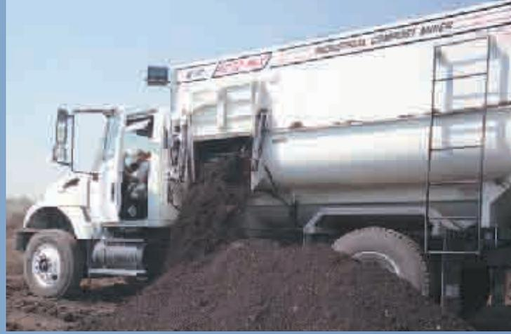
The ROTO-MIX variable rate discharge door is hydraulically operated and can be opened or closed with the mixer running to control compost flow. This feature eliminates constant PTO off-and-on, reducing torque surge and offering operation ease.
