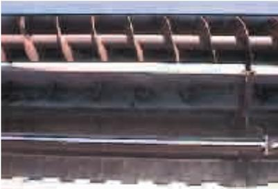
Only two augers with one-half to two-thirds less flighting than most conventional auger mixers.
