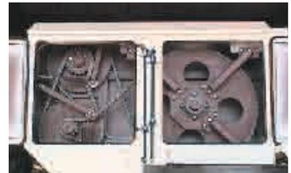
The extra heavy-duty drive assembly runs in an oil bath. A grease bank allows easy access to all drive assembly bearings.
