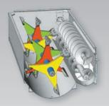
Staggered Rotor option is ideal for feeding rations that require wet distillers grains. Improved lifting and tumbling action, less revolutions, faster mix saves time and fuel and lowers maintenance costs.
