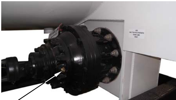
← ROTOR GEARBOX SIGHT PLUG LEVEL
