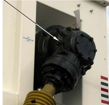
TRAILER OIL LEVEL, FILL TO THIS BOLT LEVEL
