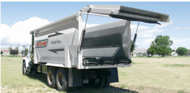
Rear Discharge - tailgate opens with two hydraulic cylinders to near 90 degrees.
